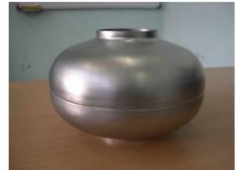
Laser welded half cells of SC Cavity at CMEL, RRCAT
