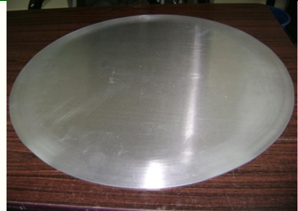
Aluminum blank, 3mm thickness
